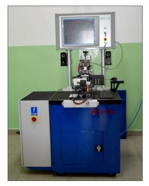
Fig. 1. MDL-54 device for measurements of ball bearing vibration levels
