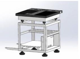
Fig. 6. Frame unit with dampers
